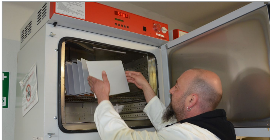
> In a safety drying chamber, a solvent-based coating on a test panel is able to dry in just one hour at 70 degrees.
