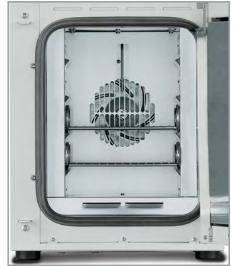
› FD 23 heating chamber with forced convection
