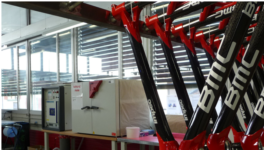
> FED and ED drying chambers are used for curing epoxy resin and epoxy adhesives
